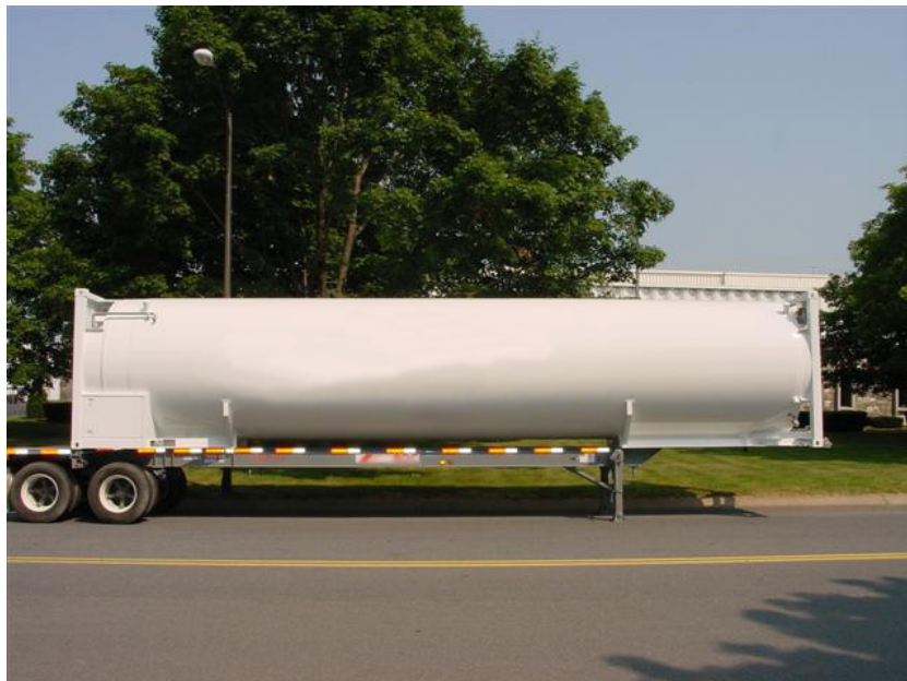
Figure C-2—Portable tank for refrigerated liquefied gas (40 ft cryogenic vacuum insulated tank container for helium with a nitrogen shield)
