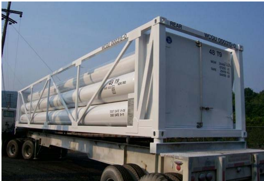
Figure C-6—Multiple element gas container (MEGC) (40 ft for compressed and liquefied compressed gas)
