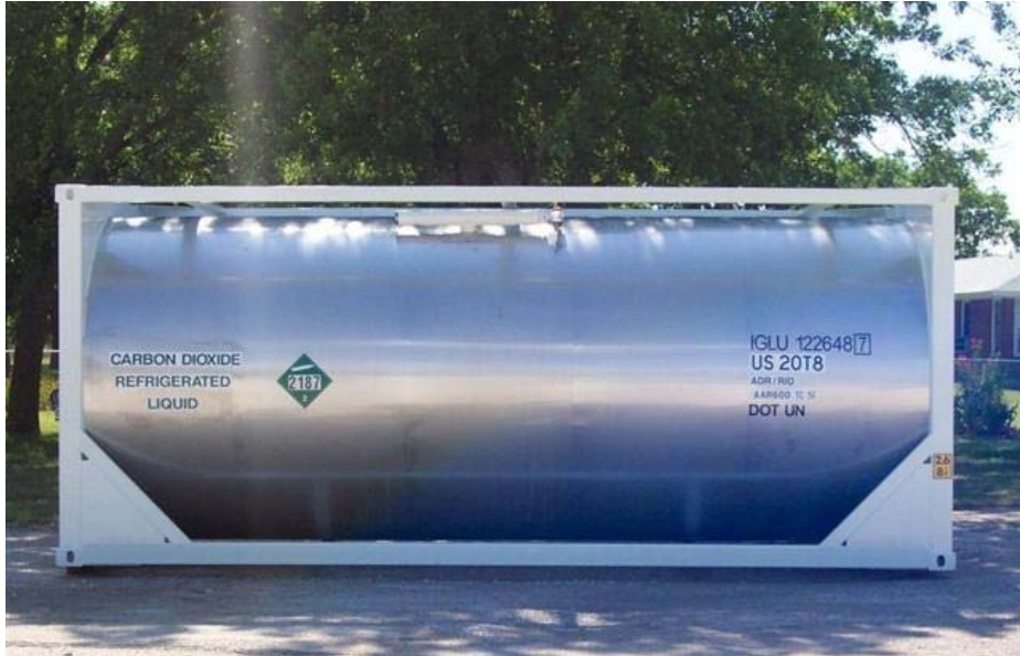
Figure C-3—Portable tank for refrigerated liquefied gas (20 ft thermally insulated tank container for carbon dioxide)
