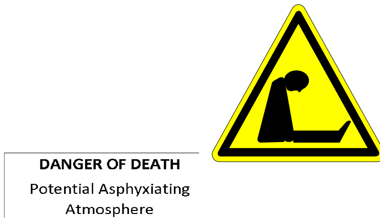
Figure 1—Example of a warning sign for asphyxiation hazard
