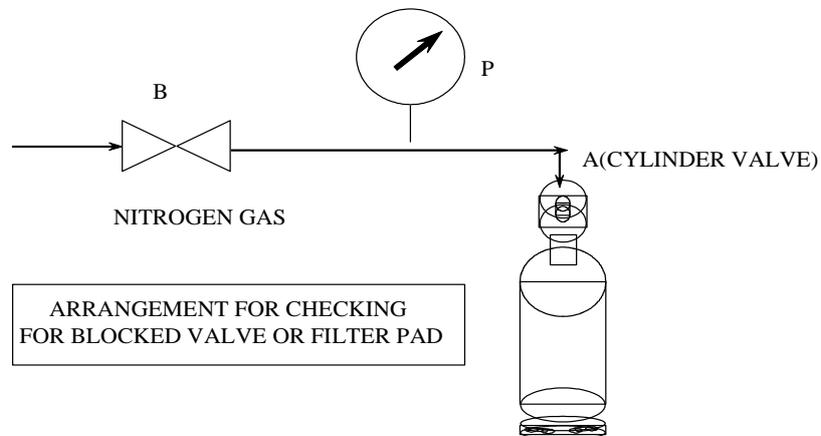
When a cylinder is found to have an obstructed gas passage in the valve, the cylinder shall be set aside and handled only by specifically trained personnel in this task. The preferred method to follow is to partially unscrew the valve within a glanded cap that is secured and joined to the cylinder and vented to a safe discharge. For further information see AIGA 025 [5].
