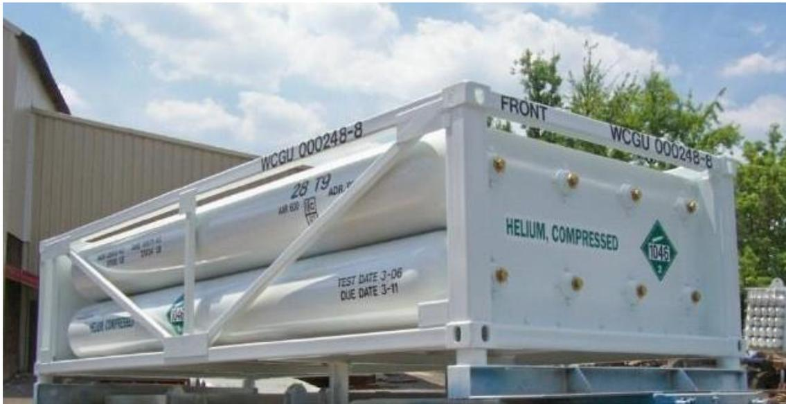
Figure A-5—MEGC (20 ft for compressed and liquefied compressed gas)
