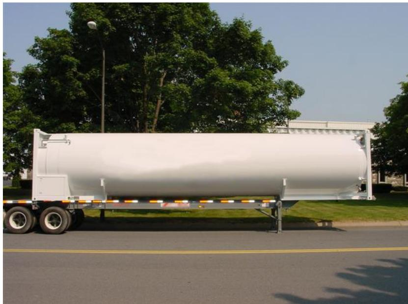
**Figure A-2—Portable tank for refrigerated liquefied gas
