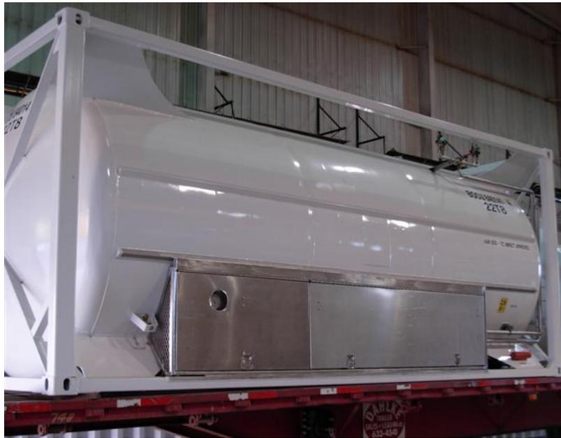
**Figure A-1—Portable tank for refrigerated liquefied gas
