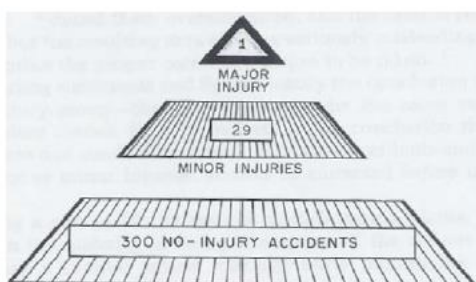
The "accident pyramid", as depicted by H. Heinrich in his 1931 book Industrial Accident Prevention: A Scientific Approach .
