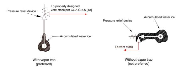
Figure 1—Typical pressure relief device installation – uninsulated cold hydrogen piping
