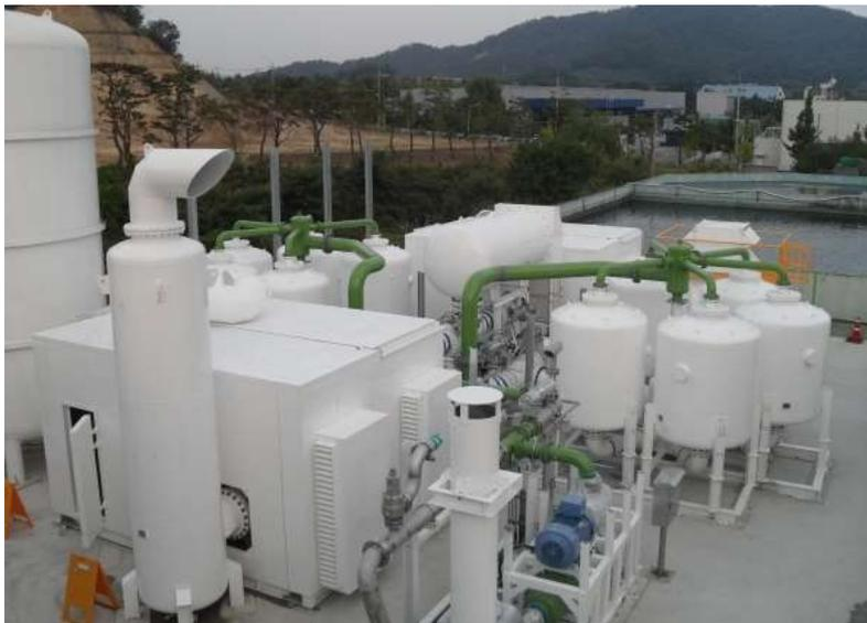
Figure 3—Example of an Oxygen VSA( Photo courtesy of Air Products and Chemicals)
