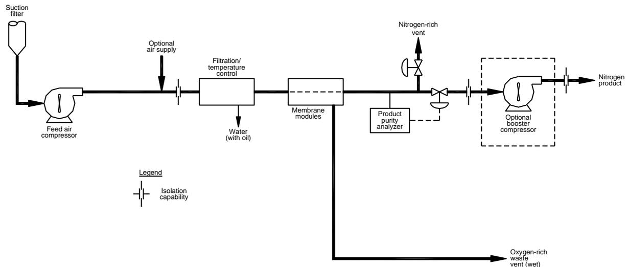
**Figure 11— Typical membrane nitrogen flow diagram**
