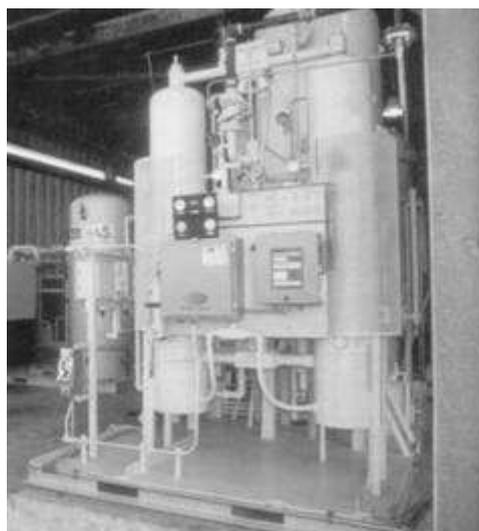
Figure 15—Example of a deoxo system
