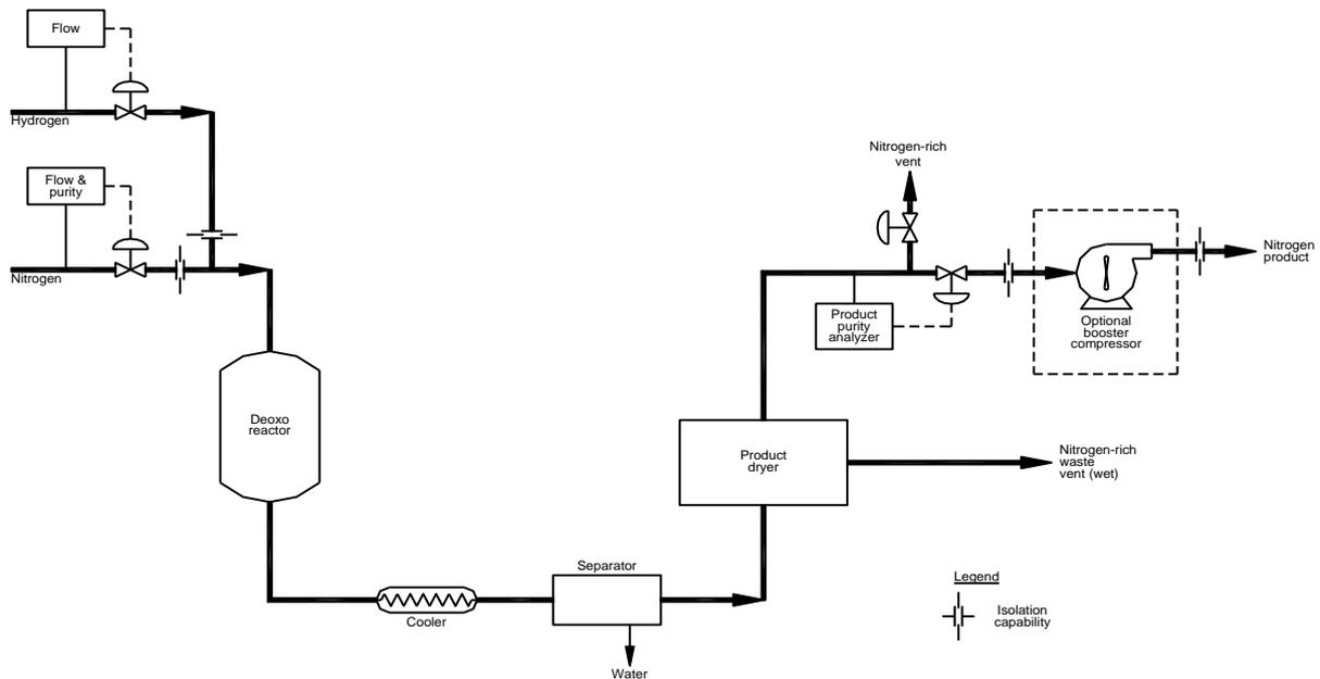
Figure 14—Typical deoxo flow diagram
