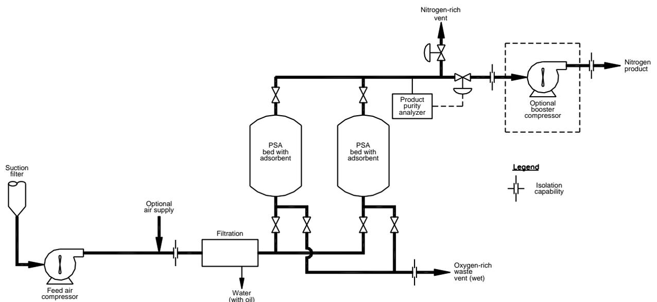
Figure 7— Typical PSA nitrogen generator flow diagram
