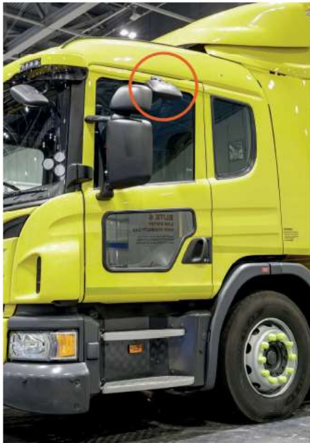
Class V mirror shall be fitted to the nearside of the vehicle
